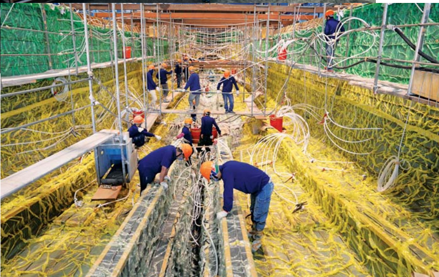
The Horizon team working on the new 6D vacuum infusion.
